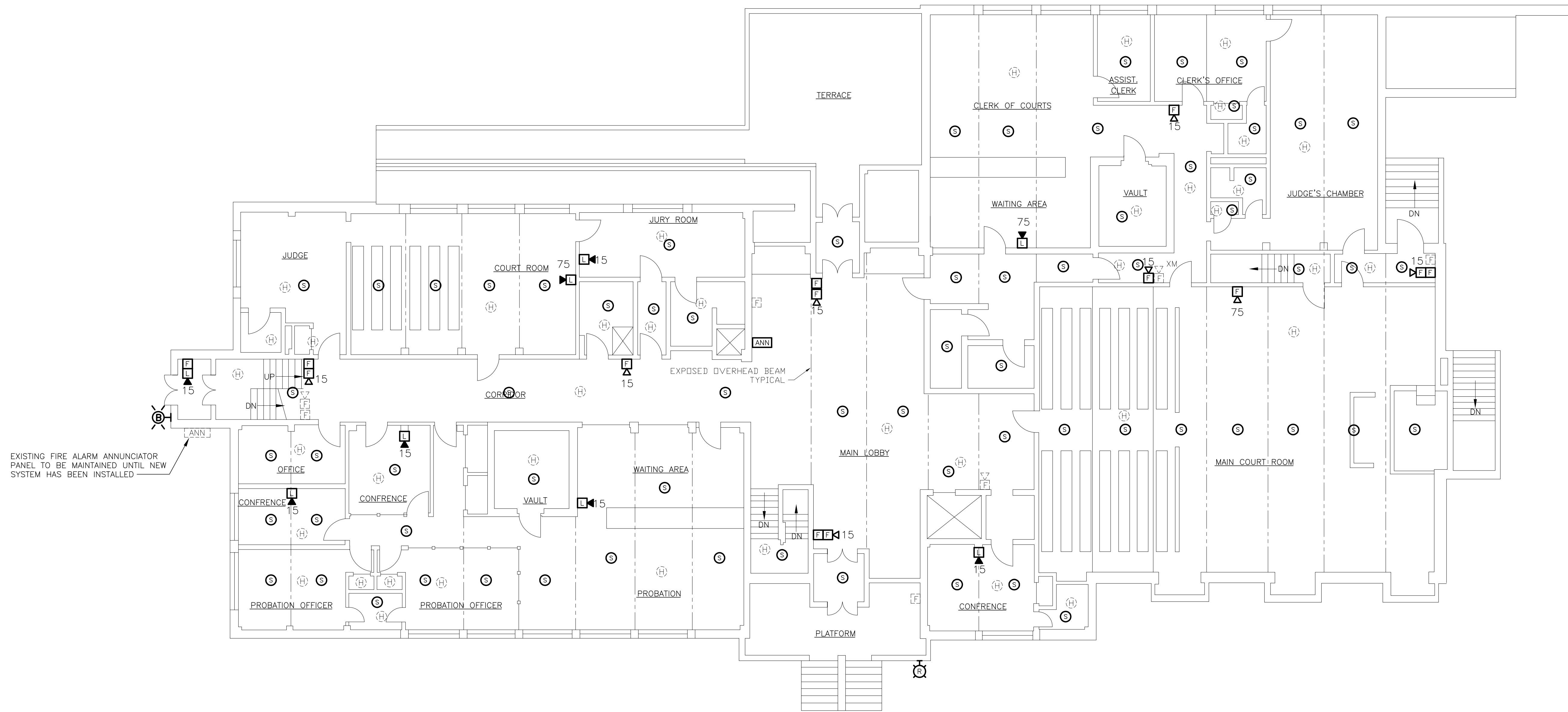
MAIN FLOOR FIRE ALARM PLAN SCALE: 1/8"=1'-0"
